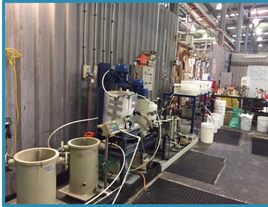
Phosphoric Acid Regeneration Circuit
