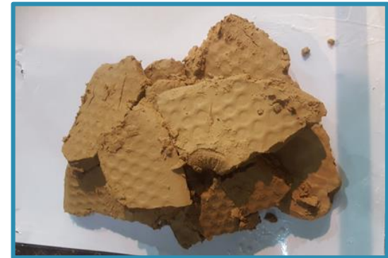
NdPr-Rich Pre-Leach Residue
