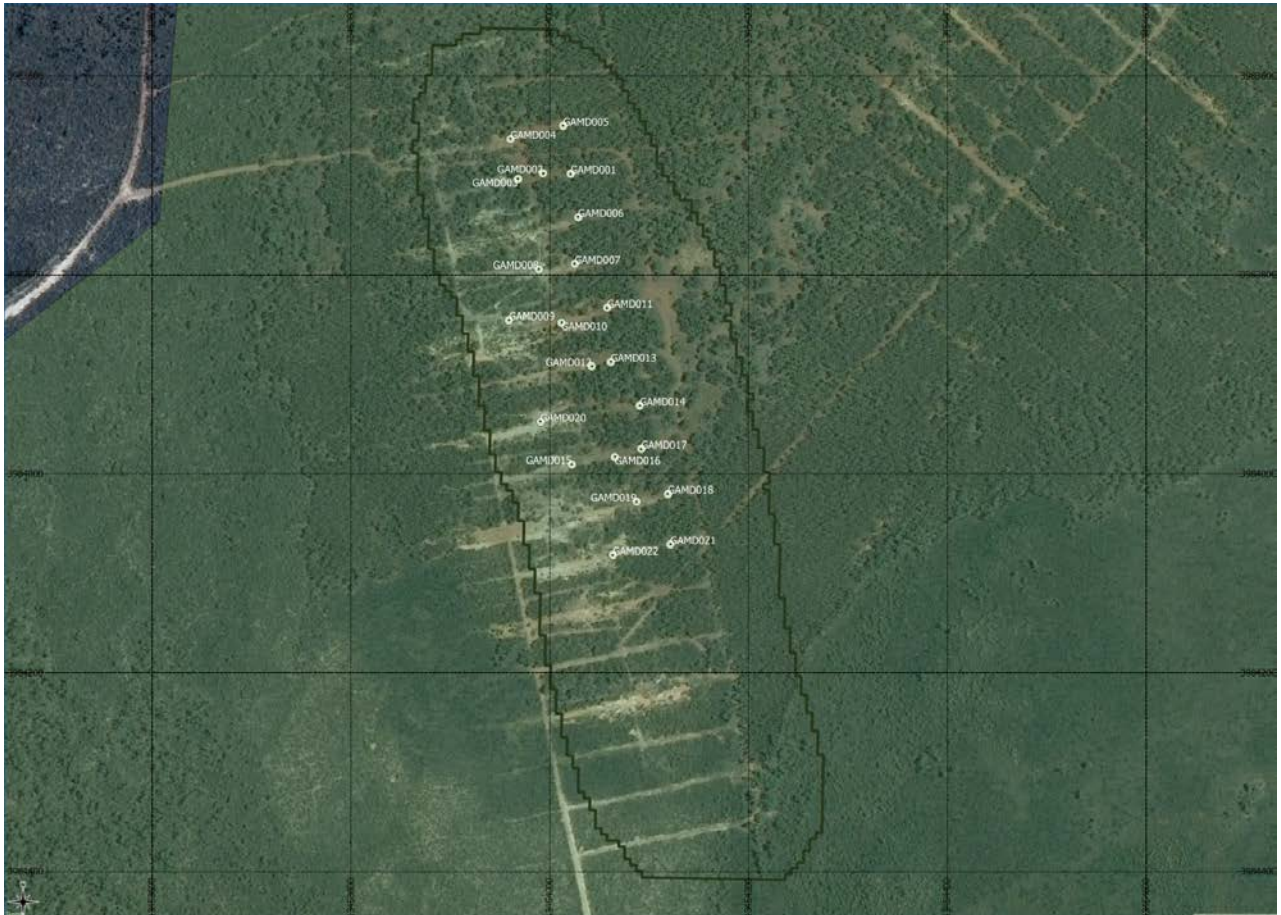
Figure 1 – Location of drill holes used to produce the metallurgical master composite and showing the proposed pit optimisation outline.
