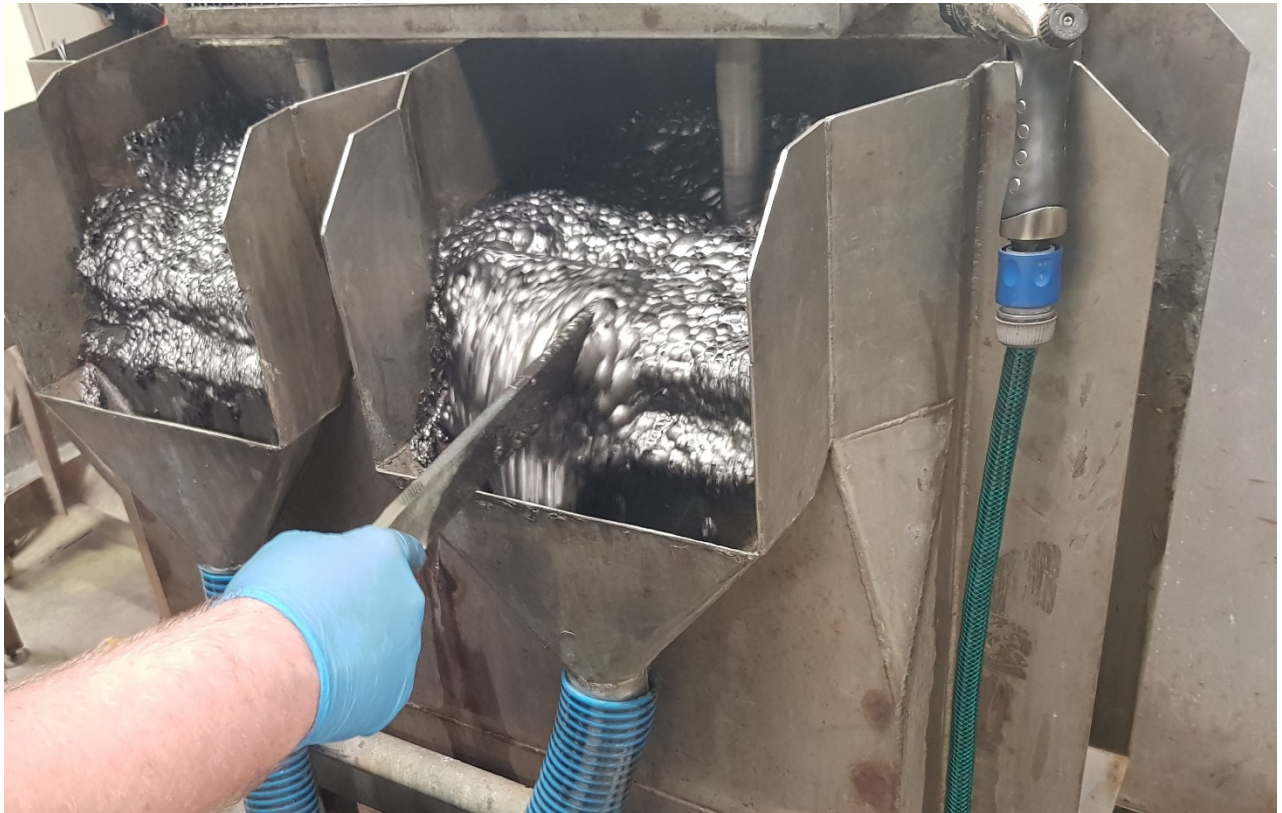
Figure 2 – Flotation on the Munglinup graphite ore during metallurgical testwork.
