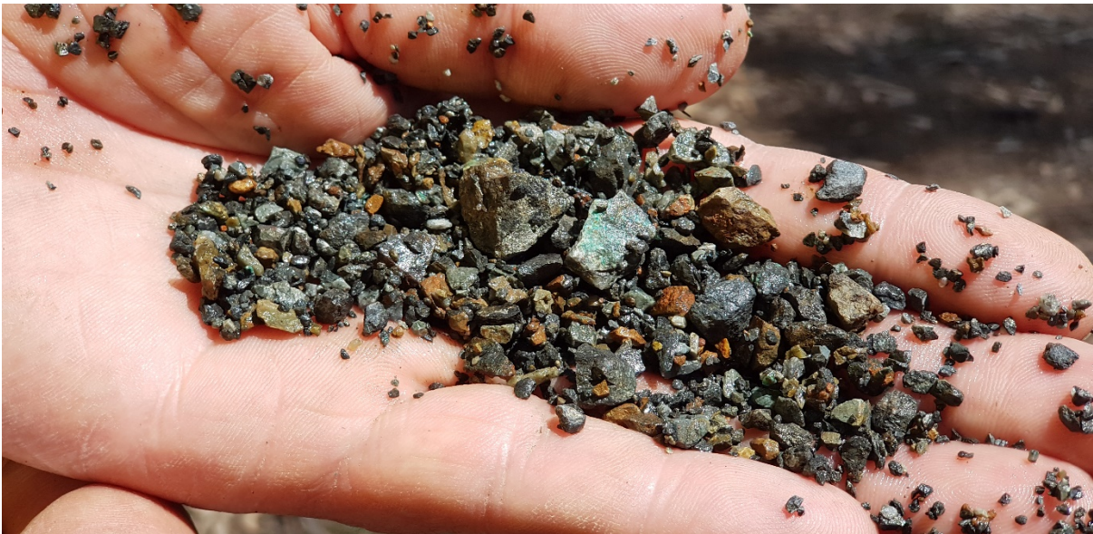
Photo 4: Oxide (malachite) & sulphide mineralisation (chalcopyrite-pyrite-pyrrhotite) occurring in drill chips (CRC004: 93 to 94m) through Sellars Lode
