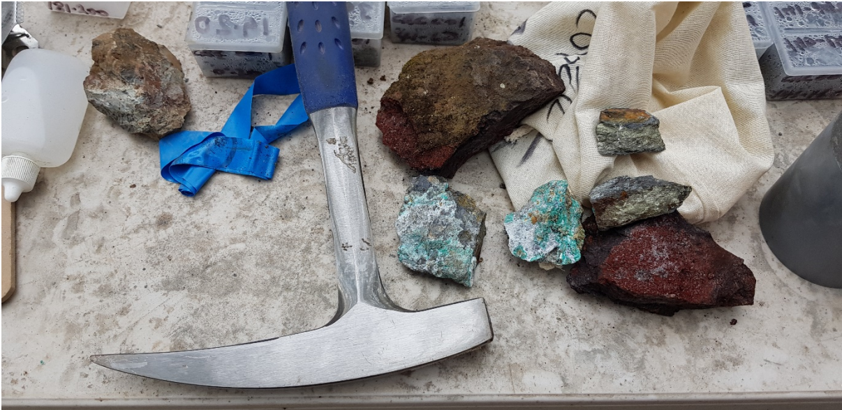
Photo 3: Selected surface gossans - copper oxide (malachite) and sulphidic rocks (chalcopyrite-pyrite-pyrrhotite) from Sellars Lode / stockpiles (refer Historical Mine Working locations at Sellars Lode on Figure 2)
