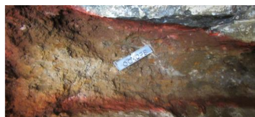
Figure 3 LEFT: Photo of samples IM-001309-11-12. Sample IM-001311 contains 33.91% Zn, 6.81% Pb and 4.5g/t Ag . INSERT BELOW: Photo of the mineralised vein at the Wari mine working at La Elegida 1. Sample IM-001078 contains 33.76% Zn, 169g/t Ag and 17.33% Pb .
