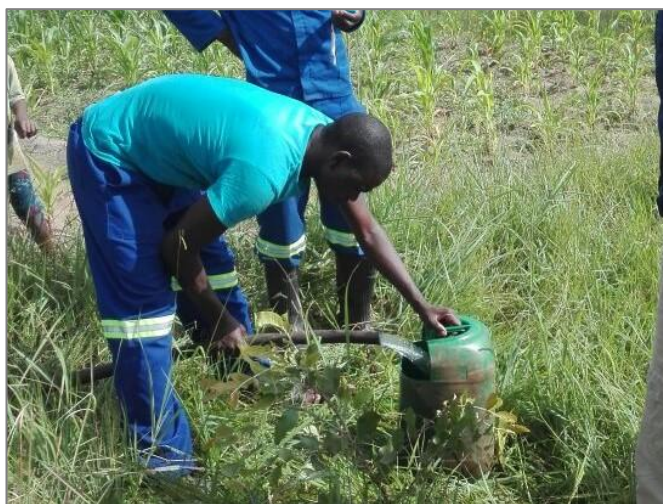
Figure 1 (LHS): Pump testing of the new hydro-monitoring wells for pit dewatering investigations at Malingunde.
