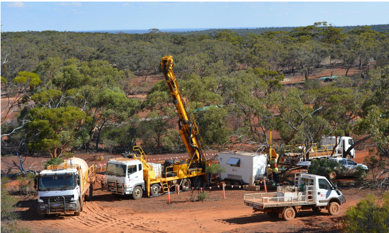
FIGURE 6 – DIAMOND RIG DRILLING AT ROTHSAY
