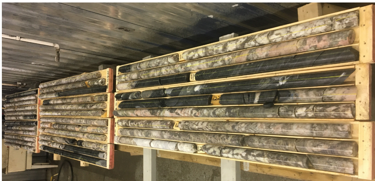
Image 1: MF18-53 intersected 68.3m of predominantly spodumene-bearing pegmatite from 82.7m.
