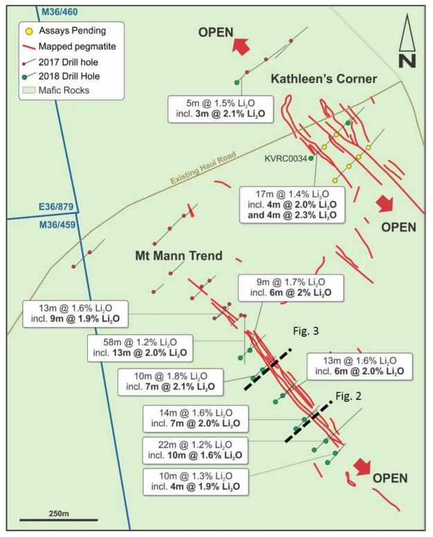
Figure 1: Kathleen Valley – Drill hole plan showing better intersections (black dashed line shows position of drill sections following)
