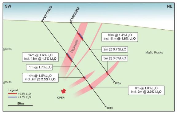
Figure 2: Kathleen Valley Project – Drill section KVRC0024 and KVRC0025 looking NW (see Figure 1 for location)
