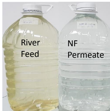
Image one: River feed (left) and Nanofiltration permeate (right)
