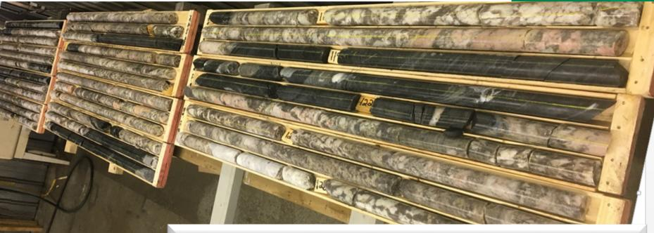
**Pioneer** RESOURCES LIMITED 2018 Drilling: Assays awaited MF18-53: 68.3m Spod Pegmatite from 82.7m MF18-57: 30m Spod Pegmatite from 117m MF18-58: 29.8m Spod Pegmatite from 116.8m MF18-51: 25.3m Spod Pegmatite from 76.7m
