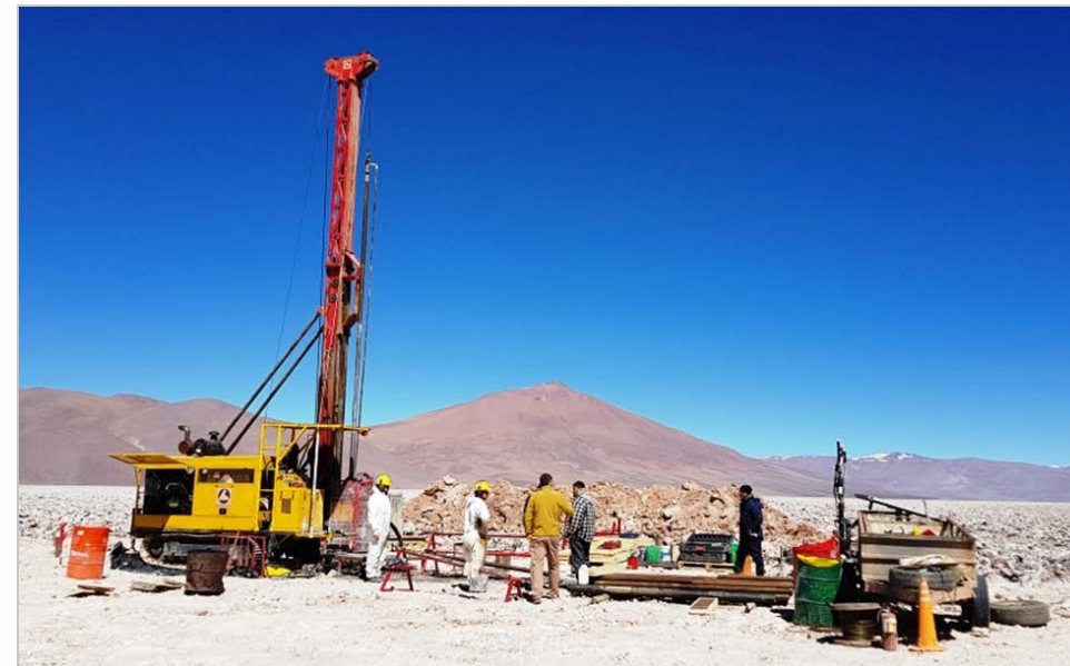
Exploration diamond drilling operations
