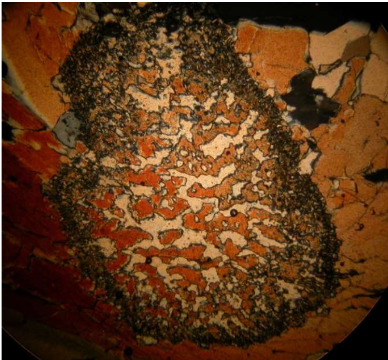
Photograph 2 Spodumene with quartz intergrowths (field of view ~3.7mm)
