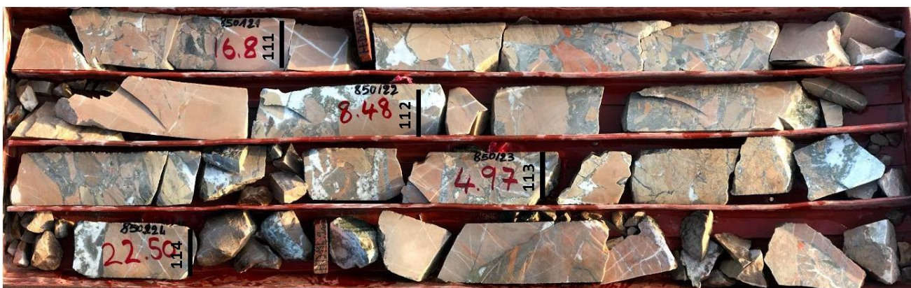
Figure 2: Diamond core from hole DDSK18-007 showing assay results (in red) from 110-114m associated with an albite-carbonate-pyrite alteration assemblage overprinting a mass flow breccia.
