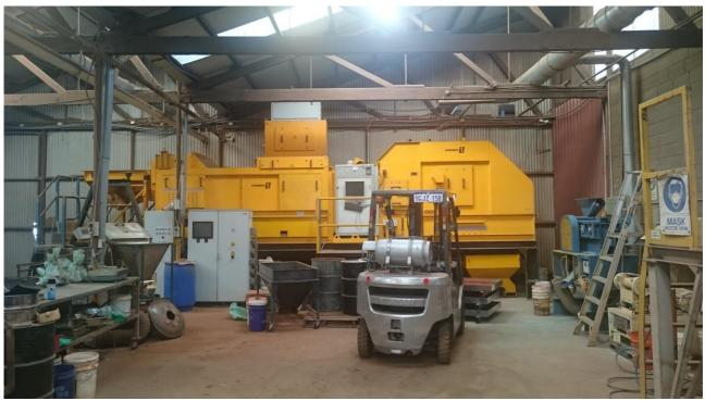
Photograph 1. Steinhert's KSS ore sorter in Perth, Western Australia.
