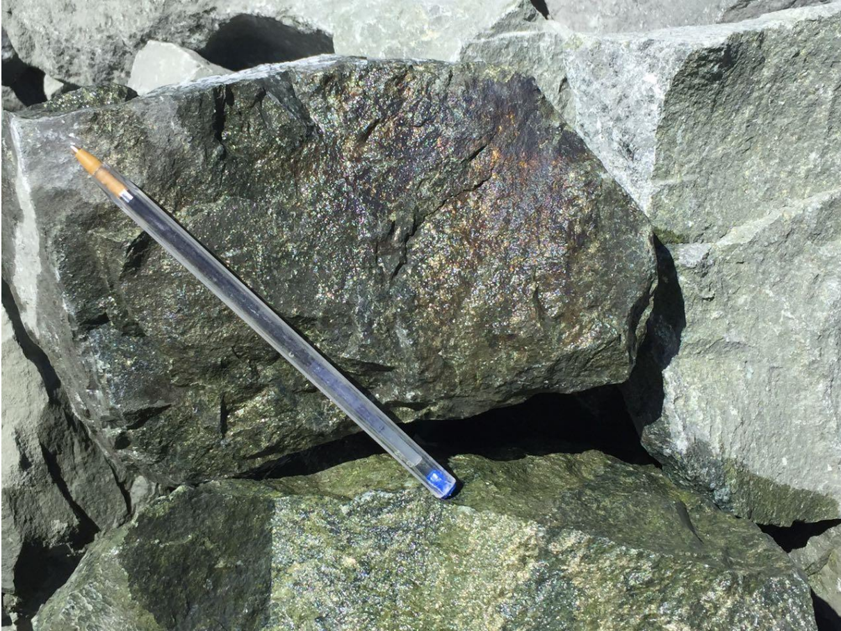
Figure 5 Ore from lease miners ROM pad at San Antonio. High grade copper is associated with chalcopyrite and bornite within a vertically intruded diorite sill.
