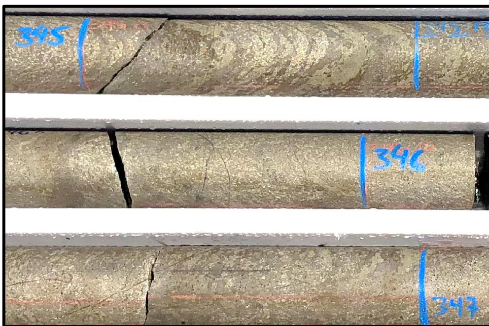
Photo 2: MDD301W1 – Close-up photo of showing massive nickel sulphides grading up to 12.60% nickel in NQ diamond core, on an open basalt contact (note the coarse-grained pentlandite crystals)
