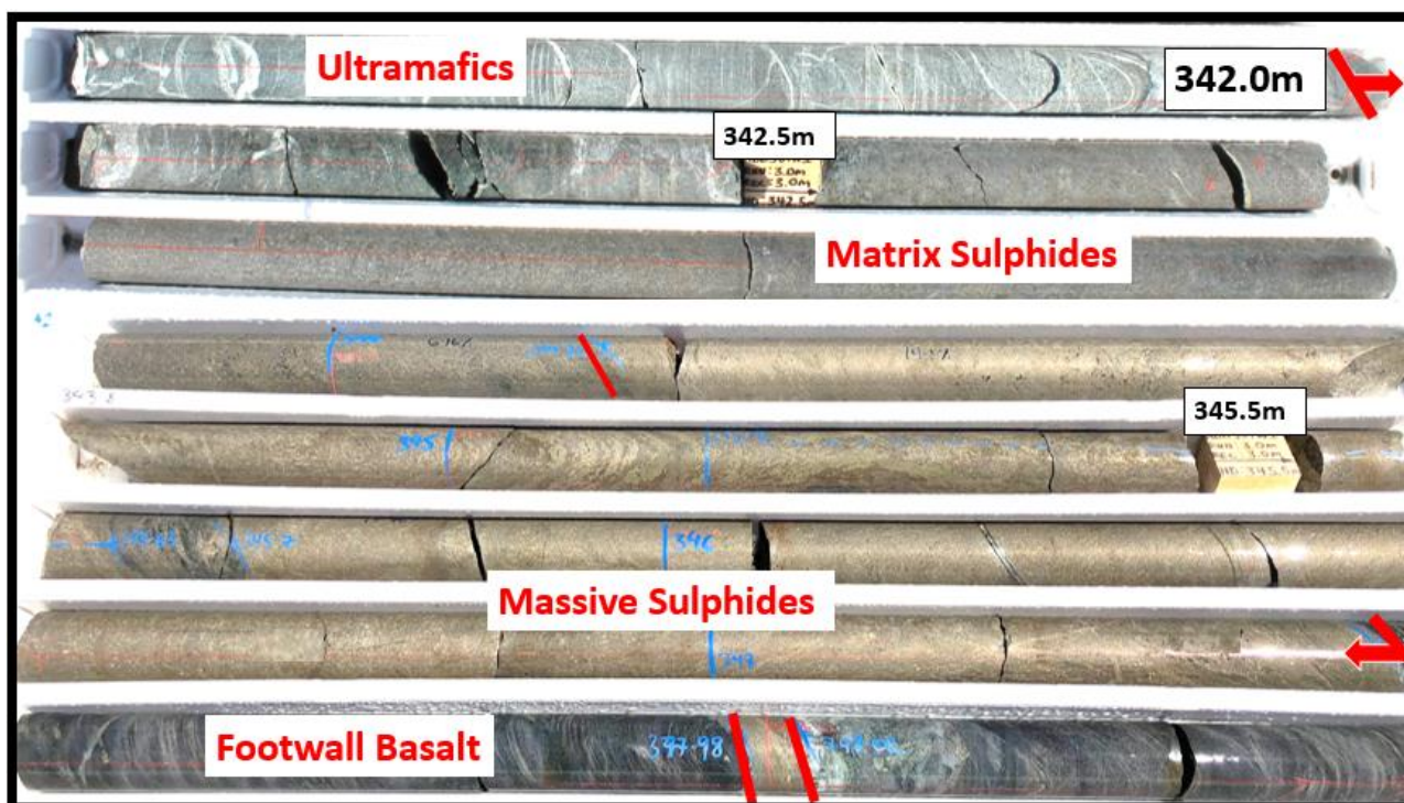
Photo 1: Impressive profile of pristine massive and matrix nickel sulphides in diamond core (MDD301W1)
