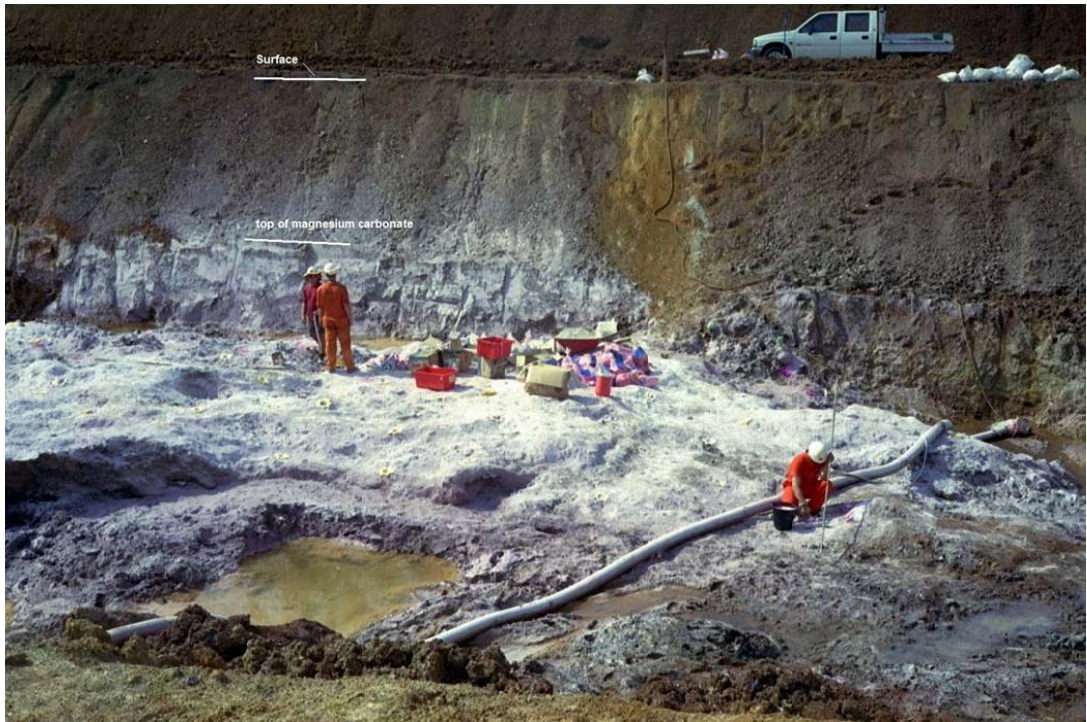
Figure 3 Test mining of magnesium carbonate rock using drill-blasting.
