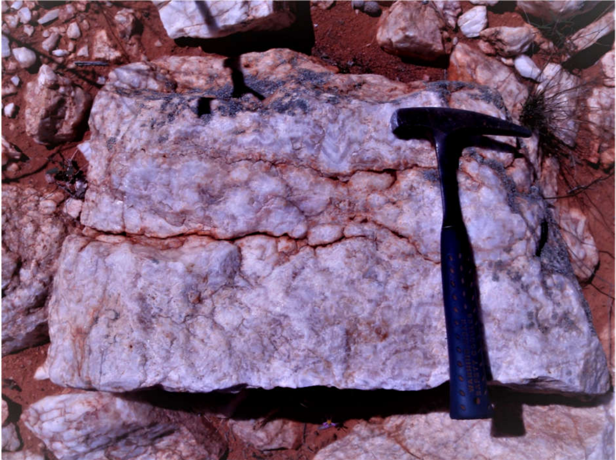
Photograph 3: Chalcedonic quartz in the Thumbo epithermal vein. The characteristic 'dogs tooth' intergrowth of crystals is common along the trend.
