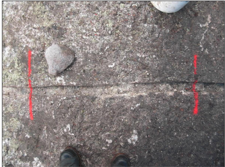
Channel sample assaying 4.94% \text{Li}_2\text{O} in drill target zone from CH16-01
