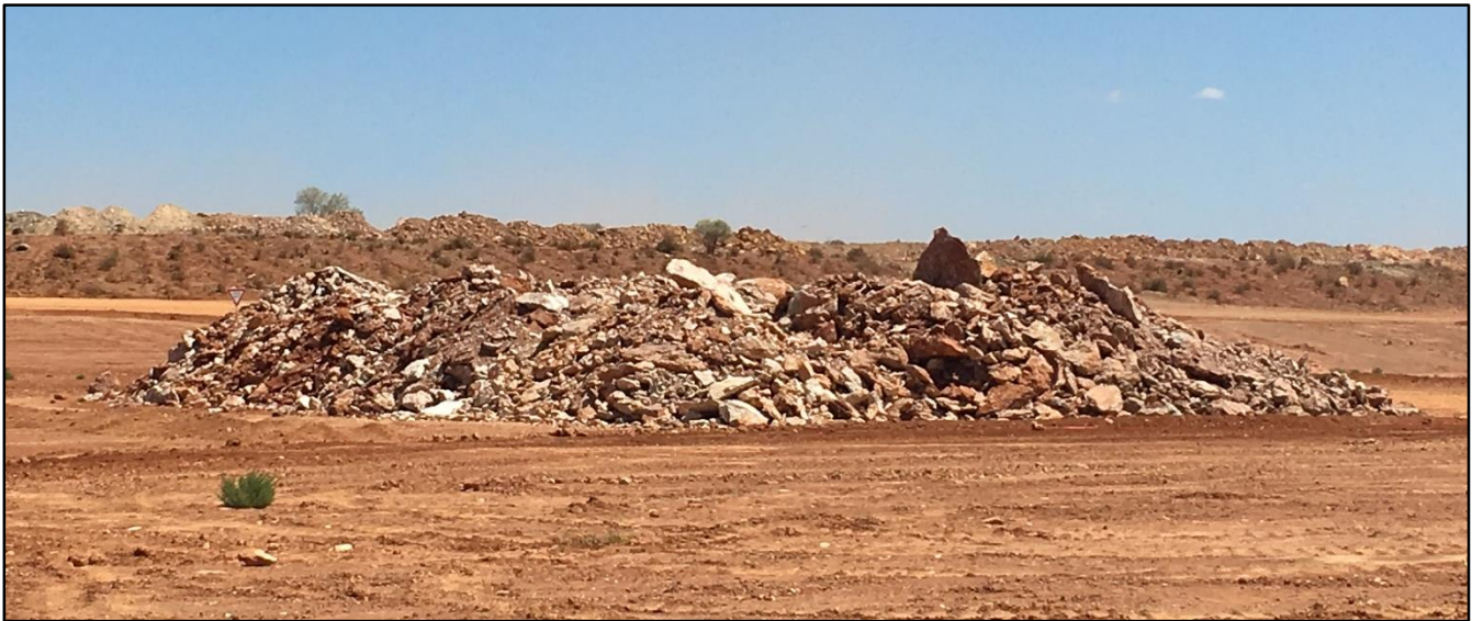
Photo 9: ROM Ore Stockpile being developed from Sly Fox, 2 months ahead of Processing
