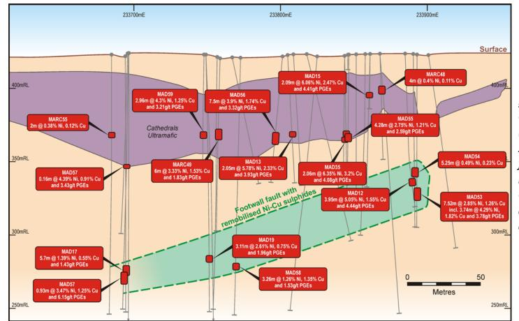
Left: a long section of the Cathedrals Prospect (looking north) showing significant intersections from both recent and historic drill holes. The Cathedrals ultramafic and footwall fault outlines are also shown.
