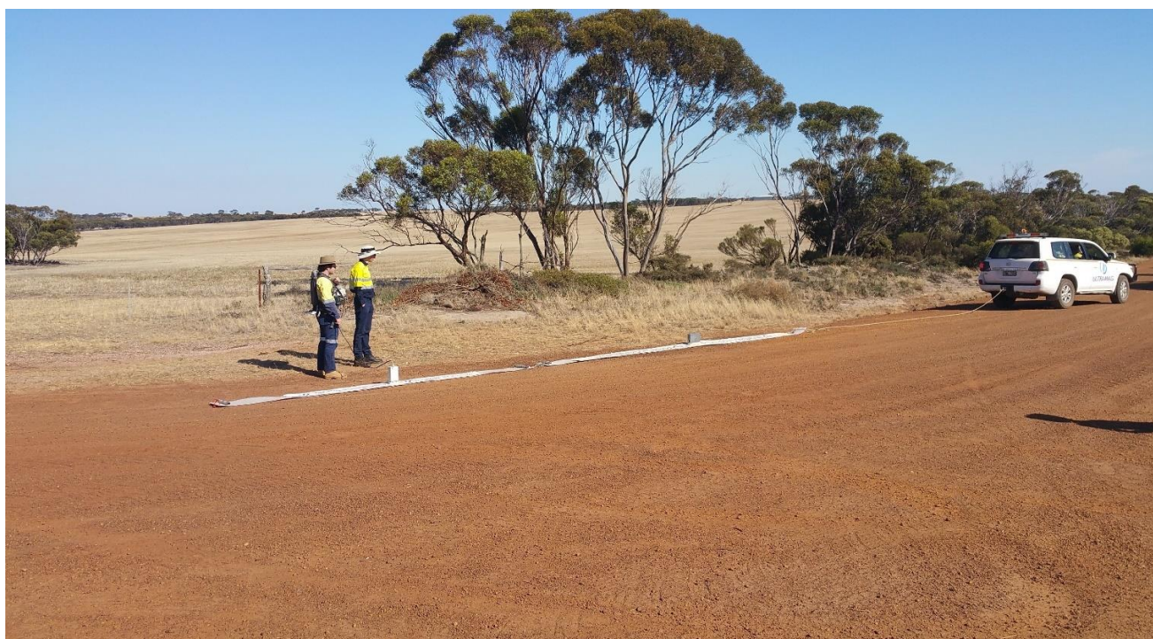
Figure 5: Typical equipment deployment, antennas, sled, transmitter and receiver.
