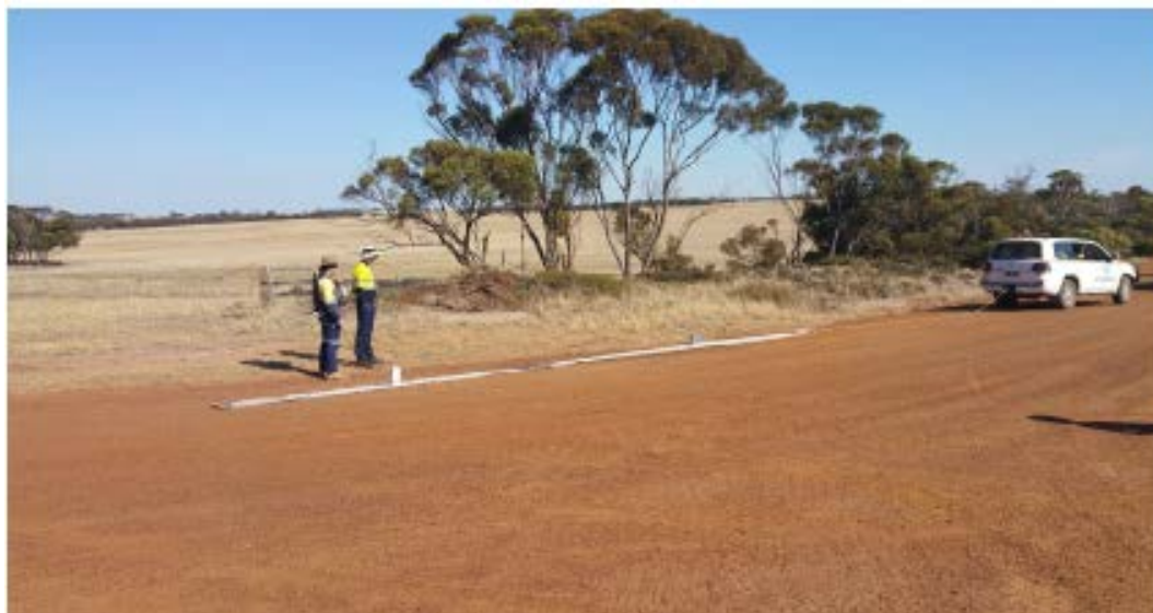
Figure 5 Ground penetrating radar survey underway
