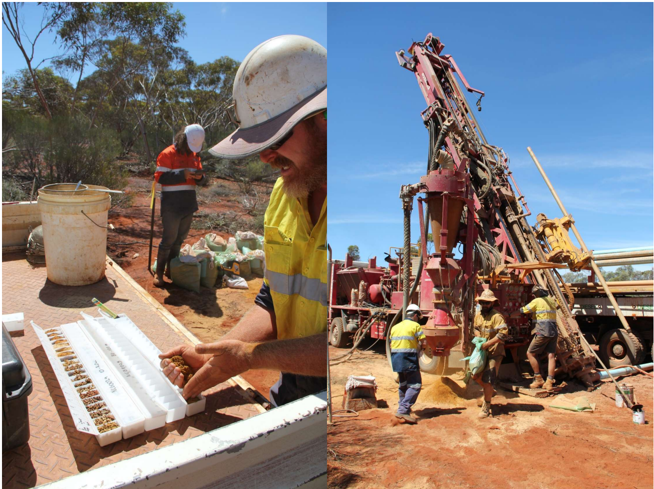
Figure 1. Reverse Circulation drilling activities at Scotia East
