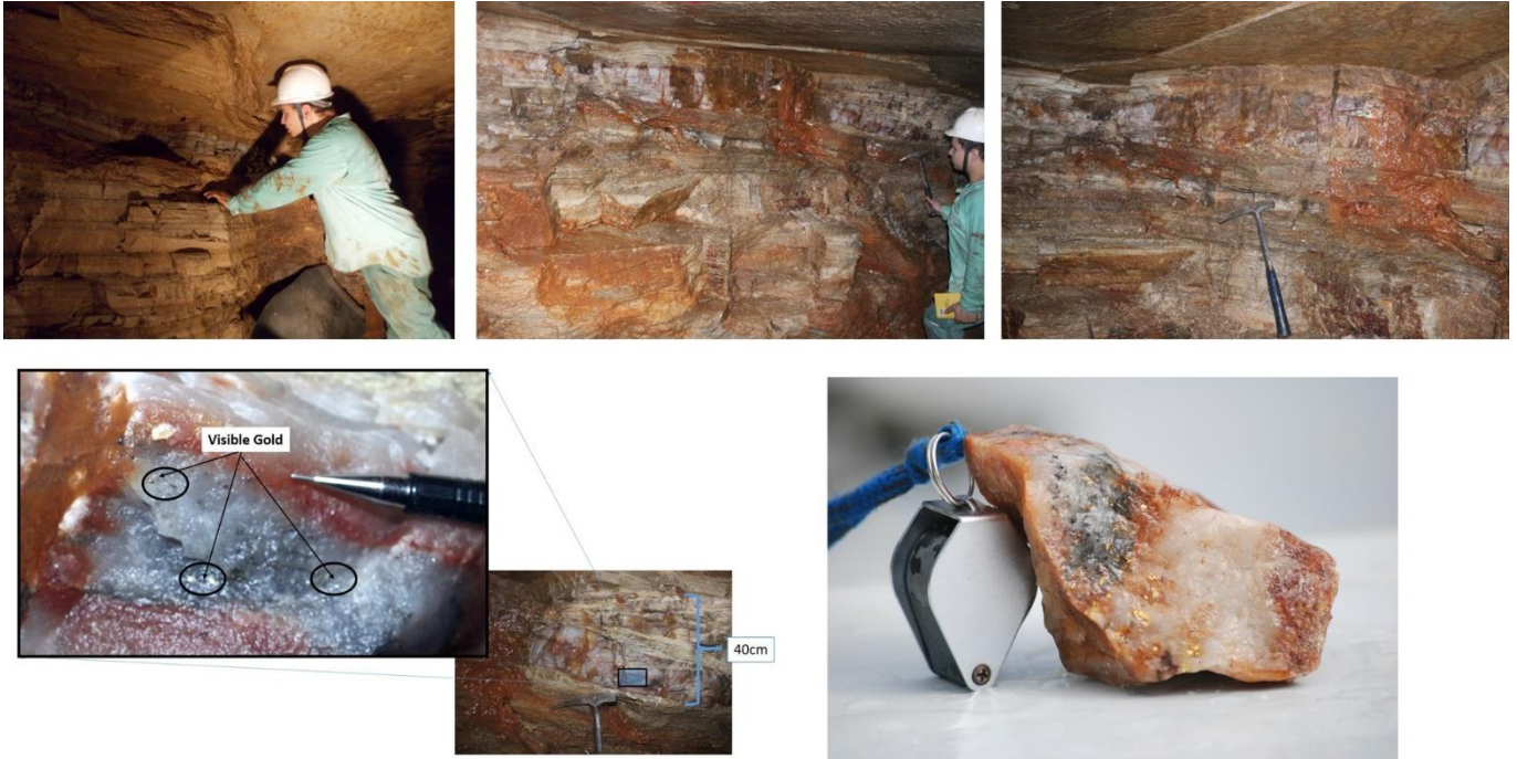
Photos- Examples of the Cuca vein on the walls of the historic workings. Visible gold constantly observed in the walls and hand samples.
