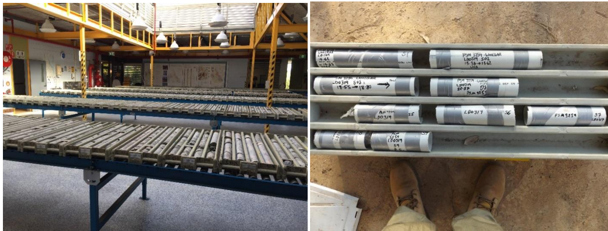
Figure 18: Left: Geotechnical drillholes laid out for scanning at the HyLogger facility in Brisbane. Right: Geotechnical samples prepared for dispatch. These are tested for mechanical strength, thus require special preparation, involving multiple layers of containment and wrapping, to avoid sustaining fractures during transport.
