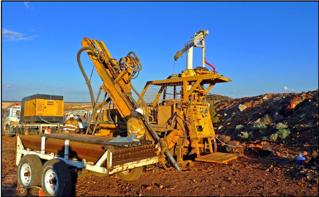
Figure 6. Specialty RC drill rig capable of drilling low-angle holes
