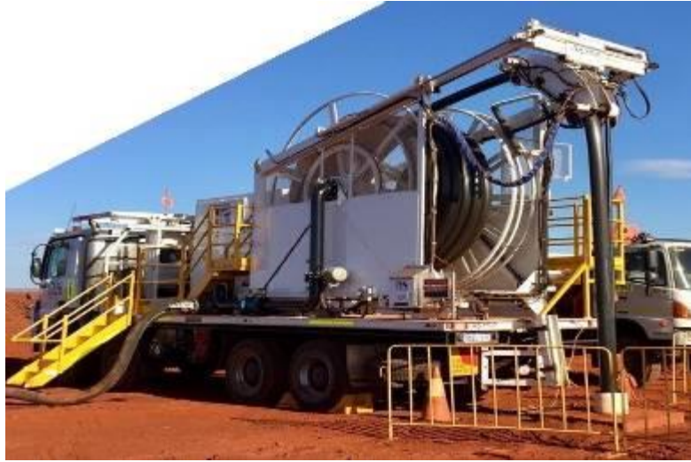
Figure 4: An example of test pumping in a Process Water Borefield
