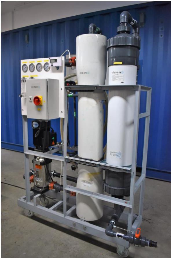
Picture: De.mem water treatment system for provision of ultraclean water to a car wash facility
