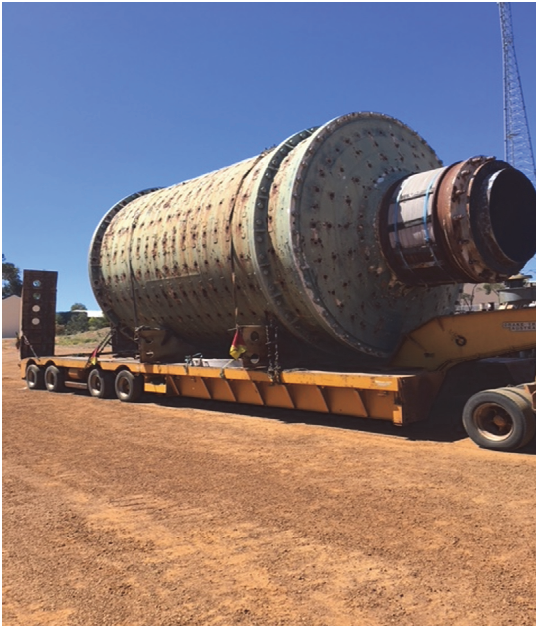
Figure 4: 25 March 2018 - Relocation of SAG Mill
