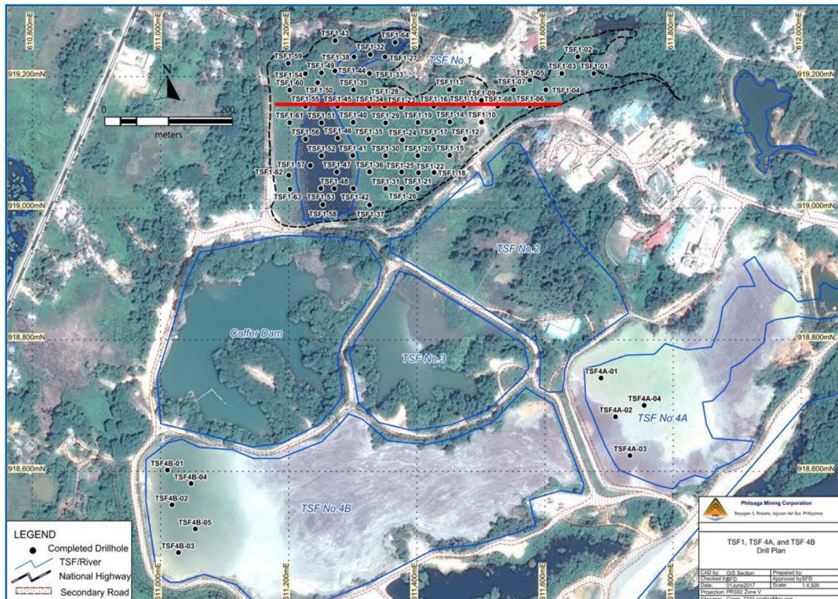
Figure 4: Location of completed drill holes in TSF 1, TSF 4A and TSF 4B.
