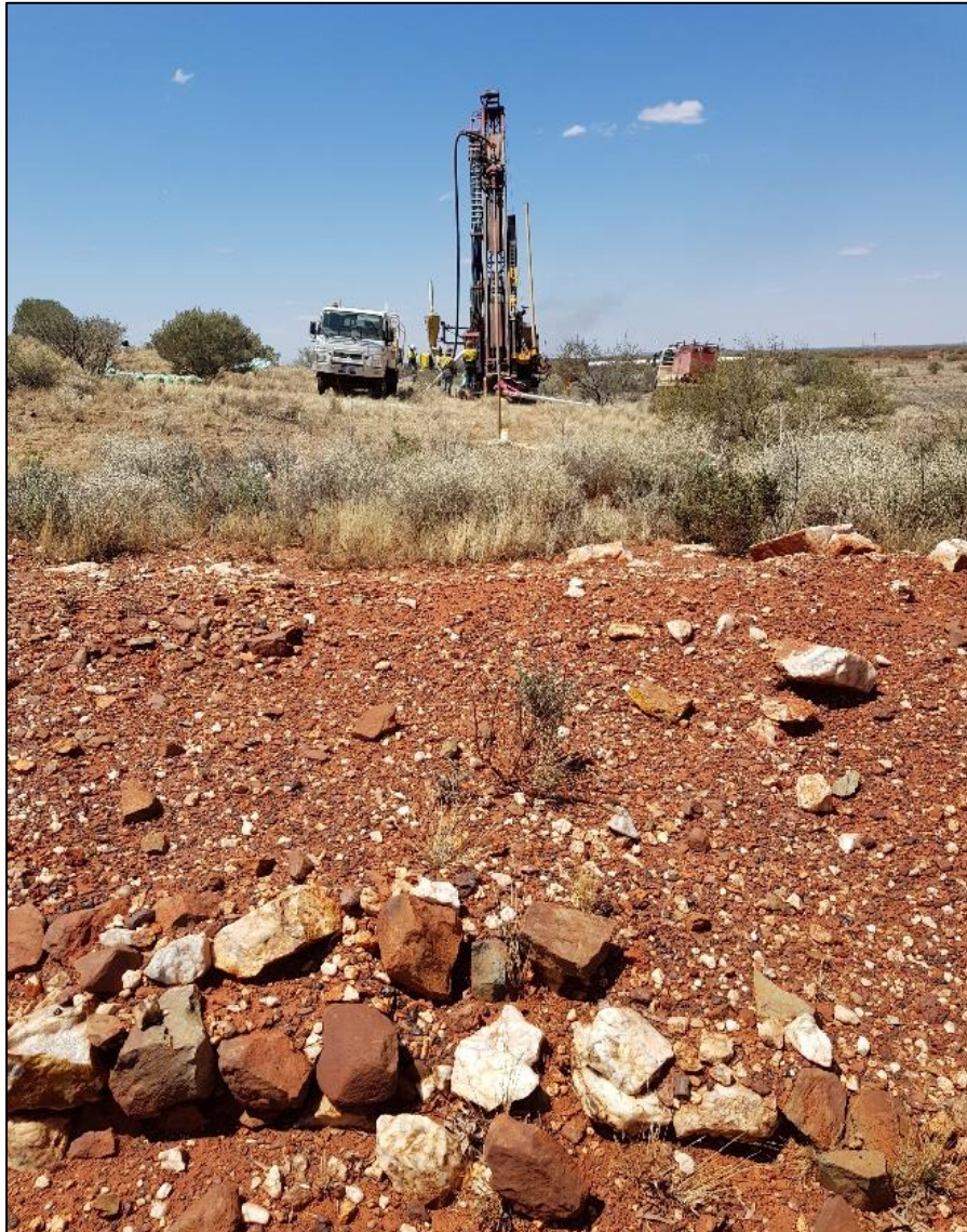
Figure 3: Photo showing RC drilling in operation at Dover Castle South.
