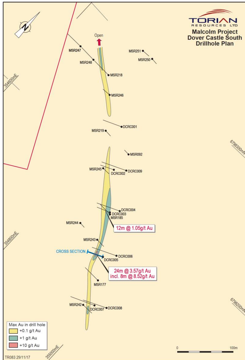
Figure 4: Drill hole plan showing gold contours at Dover Castle South (Note that recent results are 4m composites only. See Table 2 for 1m composites)
