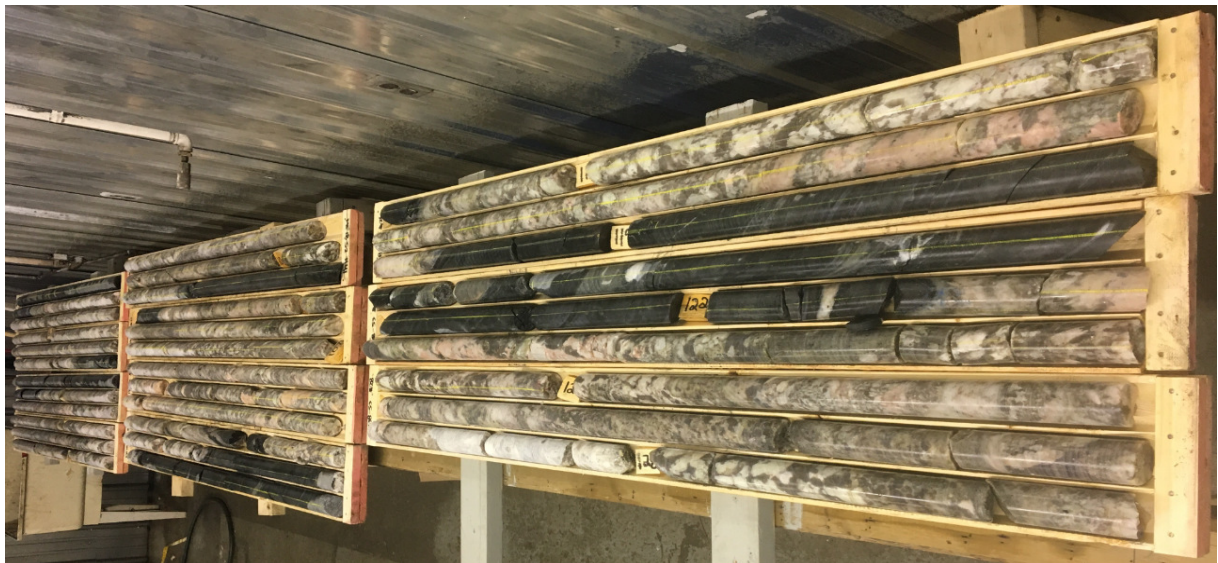
Image 1: MF18-53. The entire interval, including internal waste, returned 55.25m at 1.04% Li 2 O from 82.75m. Higher grade zones included 25m at 1.12% Li 2 O from 82.70m and 13.70m at 1.41% Li 2 O from 122.30m
