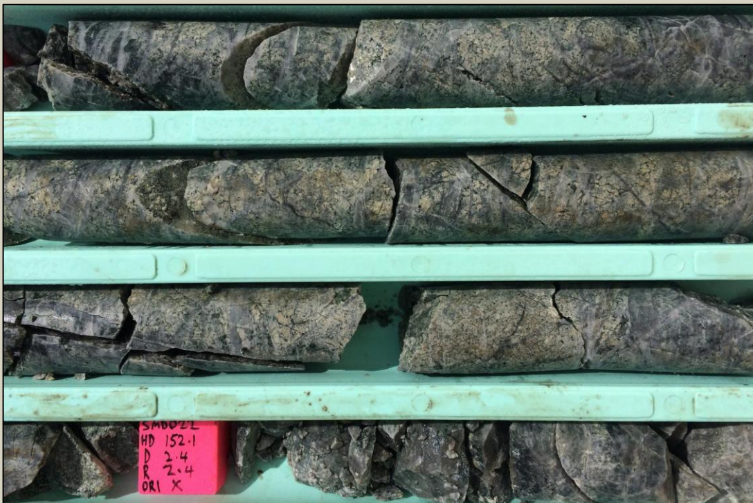
Photo 1. Porphyry 'M' veins at 152m in SMD022, similar to 'M' veining at Cadia-Ridgeway.
