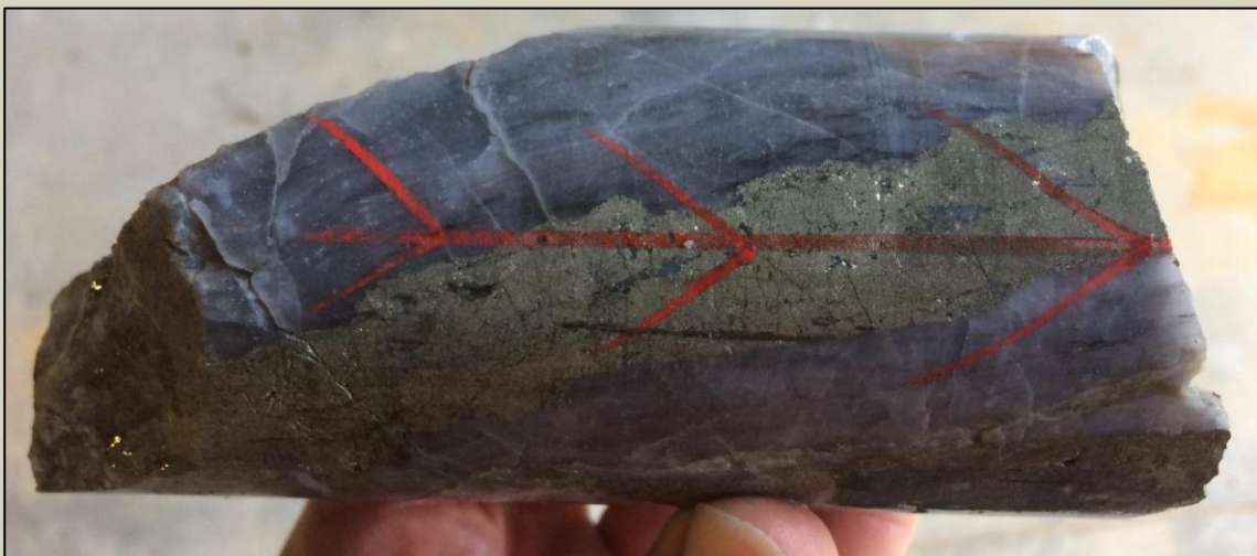
Photo 3. Laminated porphyry 'M' veins cut by pyrite 'D' vein at ~170m in SMD022.
