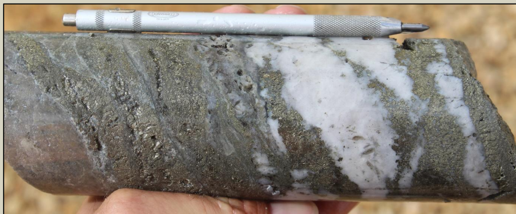
Photo 6. Quartz-pyrite-chalcopyrite 'D' vein at 235m in SMD020.
