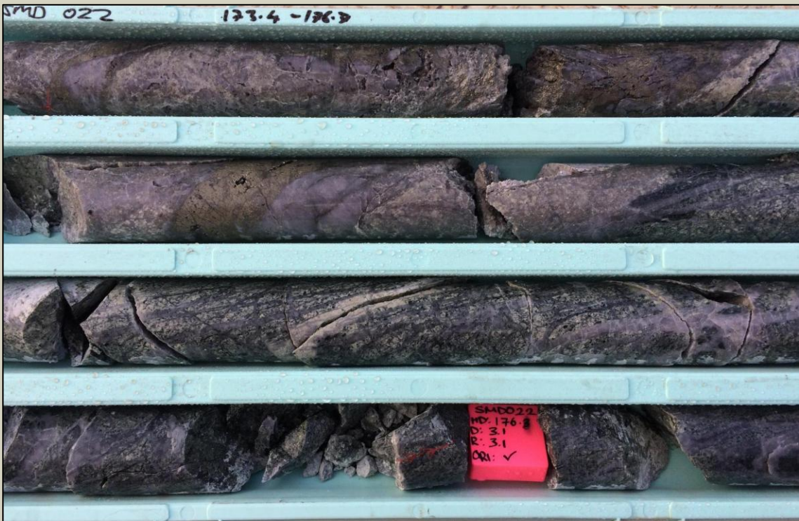
Photo 2. Porphyry 'M' veins at 176m in SMD022. The early 'M' veins (bottom 2 rows) are overprinted by later sulphide-rich 'D' veins with characteristic sericite selvages (top 2 rows).
