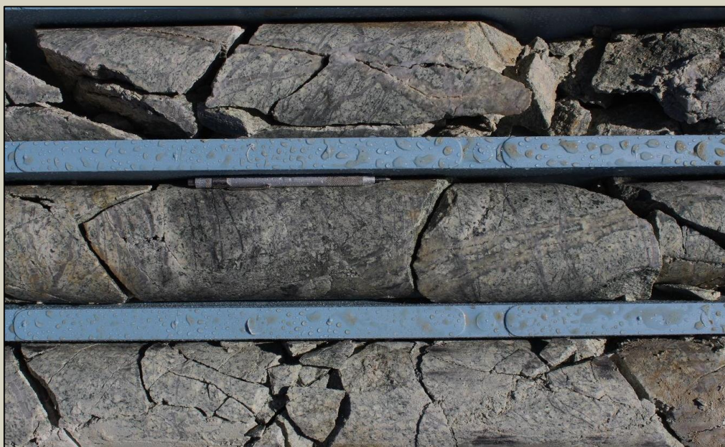
Photo 4. Quartz and quartz-magnetite stockwork veining at 88.0m in SMD019.
