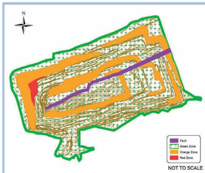
Figure 36: Geotechnical Hazard Plan (Source: Tshipi Borwa Mine)
