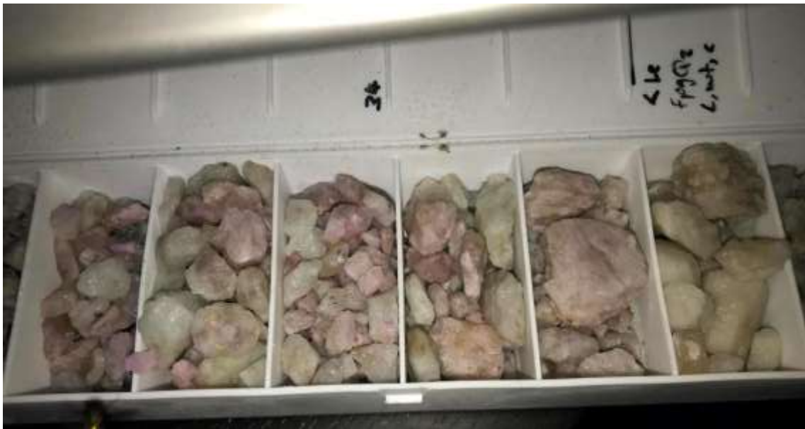
Figure 6: Spodumene-rich pegmatite chips from drill hole BDR0015.
