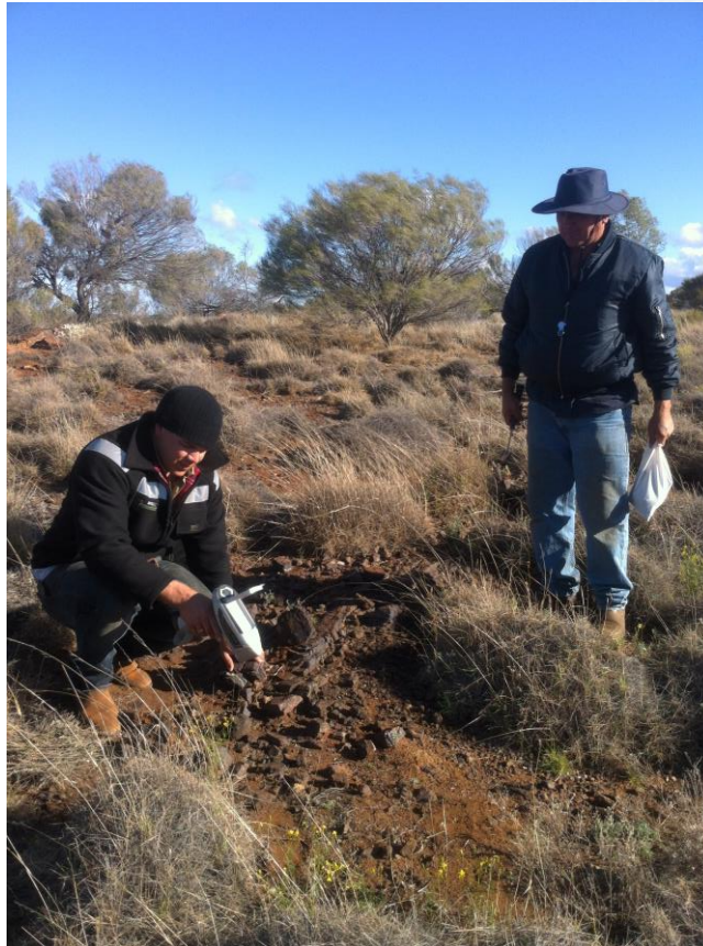
Image 1 Field sampling at Fraser Range using portable XRF
