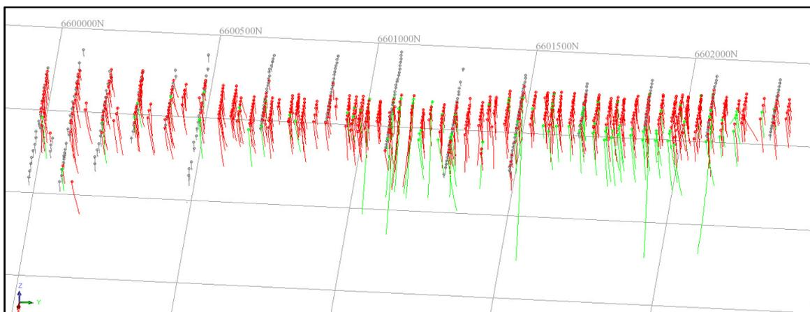
**Figure 5: Isometric view of the Bombora drilling looking downwards to the west-southwest (RC drill holes in red; diamond drill holes in green)**
