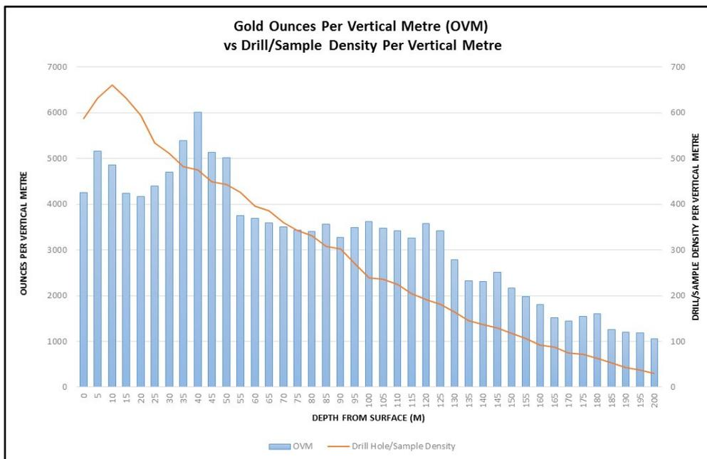
**Figure 4: Bombora Mineral Resource – OVM vs drill/sample density with depth as measured by the number of drill samples sorted by depth (RL) increments**
