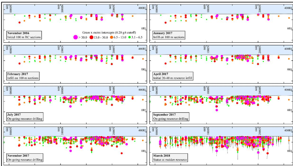
**Figure 2: Time lapse depiction of progress of Bombora drilling in long section (downhole drill hole intersections colour-coded by gram x metre)**
