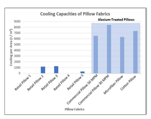
The results of the testing provided a measurement using Joules per gram (J/g), detailing the specific amount of heat being absorbed for each PCM-treated fabric. The resulting enthalpic cooling, or cooling capacity, was therefore determined for each PCM-treated pillow fabric. The results, using this measuring protocol, show that Alexium Alexicool-treated pillows compare very favourably against other similar products available on the market.
