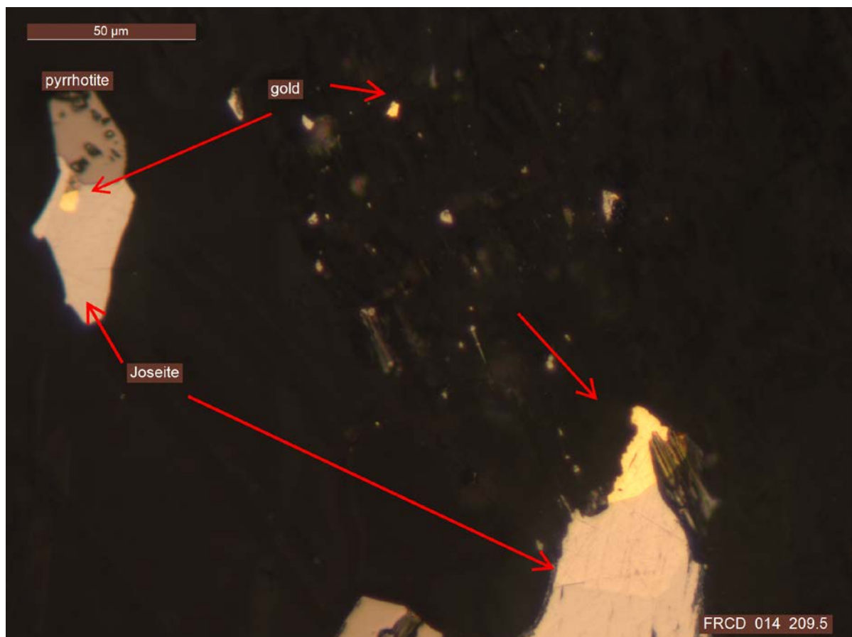
Figure 3 - Think Big - Primary Bed Rock Mineralisation – Polished Section of Drill Core Showing Native Gold
