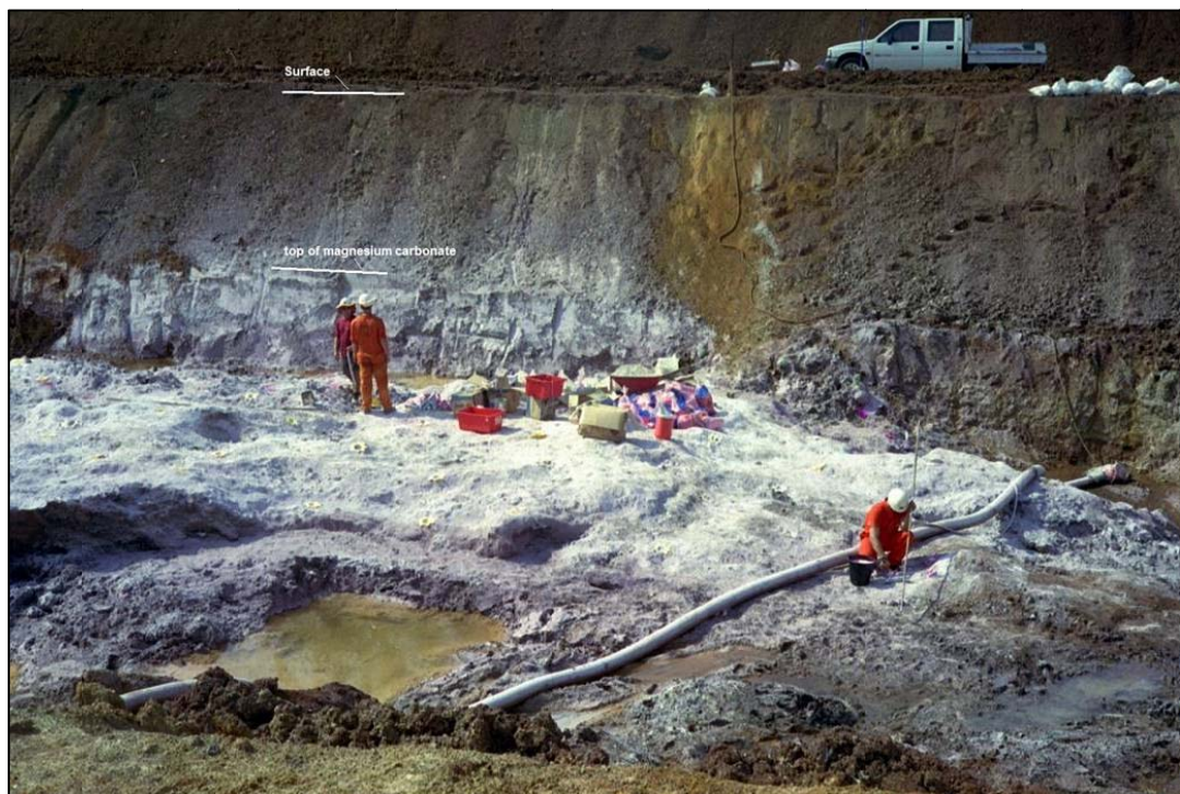
Figure 1 Test mining of magnesium carbonate rock at Winchester project (setting of explosives)
