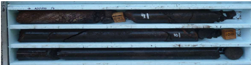
Photograph - Massive MnO mineralisation in ADD006 (part 8.80m to 12.00m) Significant intersection of brecciated and massive manganese mineralisation (up to 62.18% MnO).
