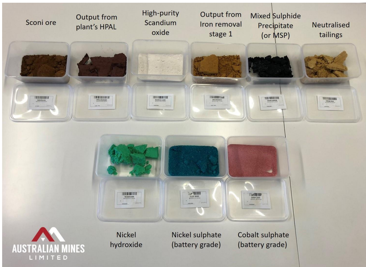
Figure 4: Samples taken from the various stages of Australian Mines' demonstration plant in Perth, Australia. The top row is considered by Australian Mines as the 'front end' of the plant, with the bottom row considered the 'back end' of the plant.
