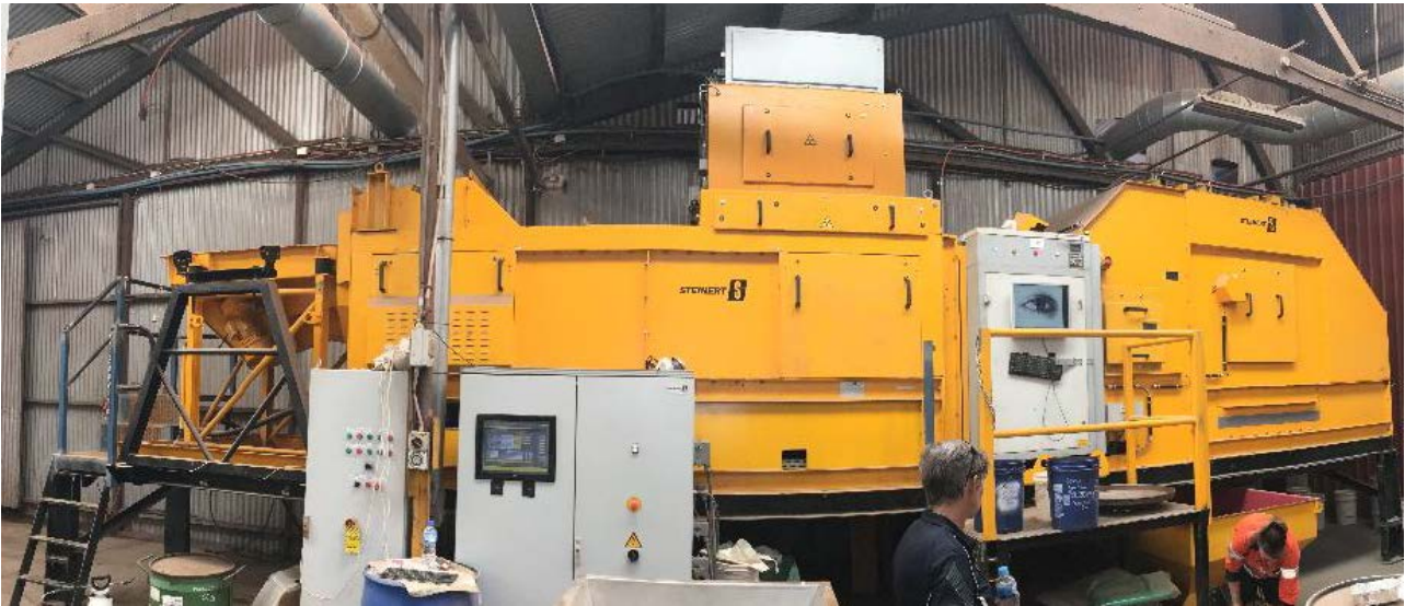
FIGURE 9 – STEINERT MULTI-SENSOR ORE SORTER AT NAGROM IN WESTERN AUSTRALIA
