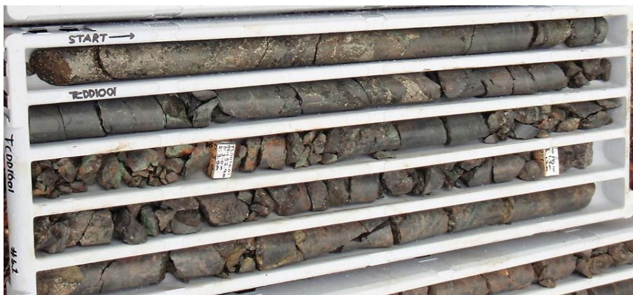
Photo 2: TCDD001 drill core from 151.1m to 154.9m
