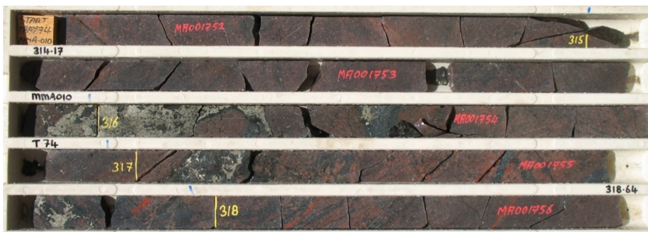
Figures: FC2 Prospect, MMA010 drill hole. Cross-section showing ~100 m interval of anomalous Cu-Co-Ni mineralisation at base of hole correlating with increased IP chargeability (top). Cut core showing interval 314.17m – 318.64m DH. Note pyrite, actinolite, chlorite & chalcopyrite veins in an albite-altered host. Assays for the interval from 315 to 318m DH averaged 0.26 wt % Cu, 521ppm Co and 905ppm Ni (bottom).
