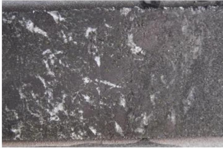
Figure 6. Large graphite flakes halved graphitic schist from MODD 015
