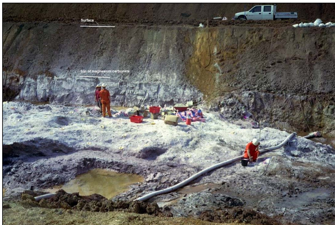
Figure 3 Test mining of magnesium carbonate rock at Winchester project showing top of mineralisation and thickness of overburden.
