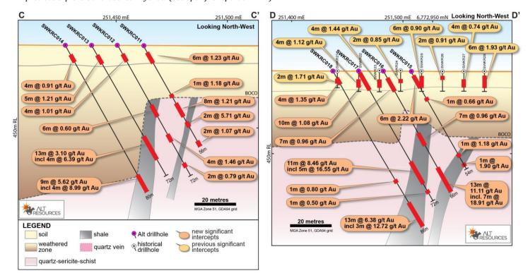
Figure 3. Cross-sections C-C' and D-D' for the first modern drilling at Southwark, Bottle Creek. The location of sections is shown in the plan map in Figure 4. Alt's new drilling results from this announcement are labelled in orange, whilst historical intercepts from previous explorers are labelled in yellow (See open file report a 28505).
