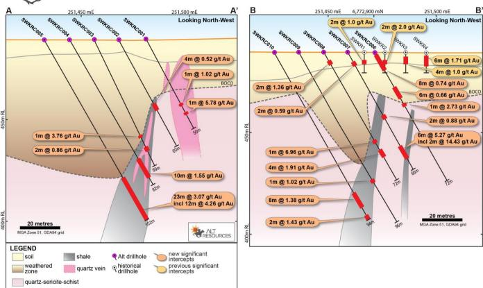
Figure 2. Cross-sections A-A' and B-B' for the first modern drilling at Southwark, Bottle Creek. The location of sections is shown in the plan map in Figure 4. Alt's new drilling results from this announcement are labelled in orange, whilst historical intercepts from previous explorers are labelled in yellow (See open file report a28505).
