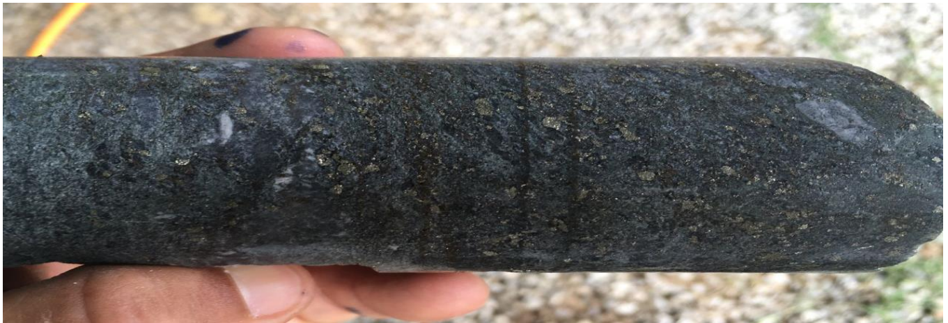
Photo 3: Detail of the sericitic alteration, with ASPY and PY in the impure limestone at ANT_004, 154m depth
