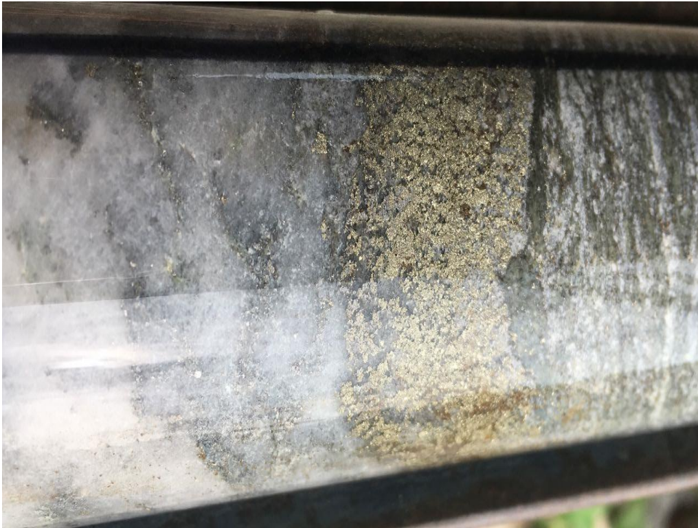
Photo 1: Core showing sericitic alteration, with ASPY and PY in a quartz vein at ANT_004, 159m depth
