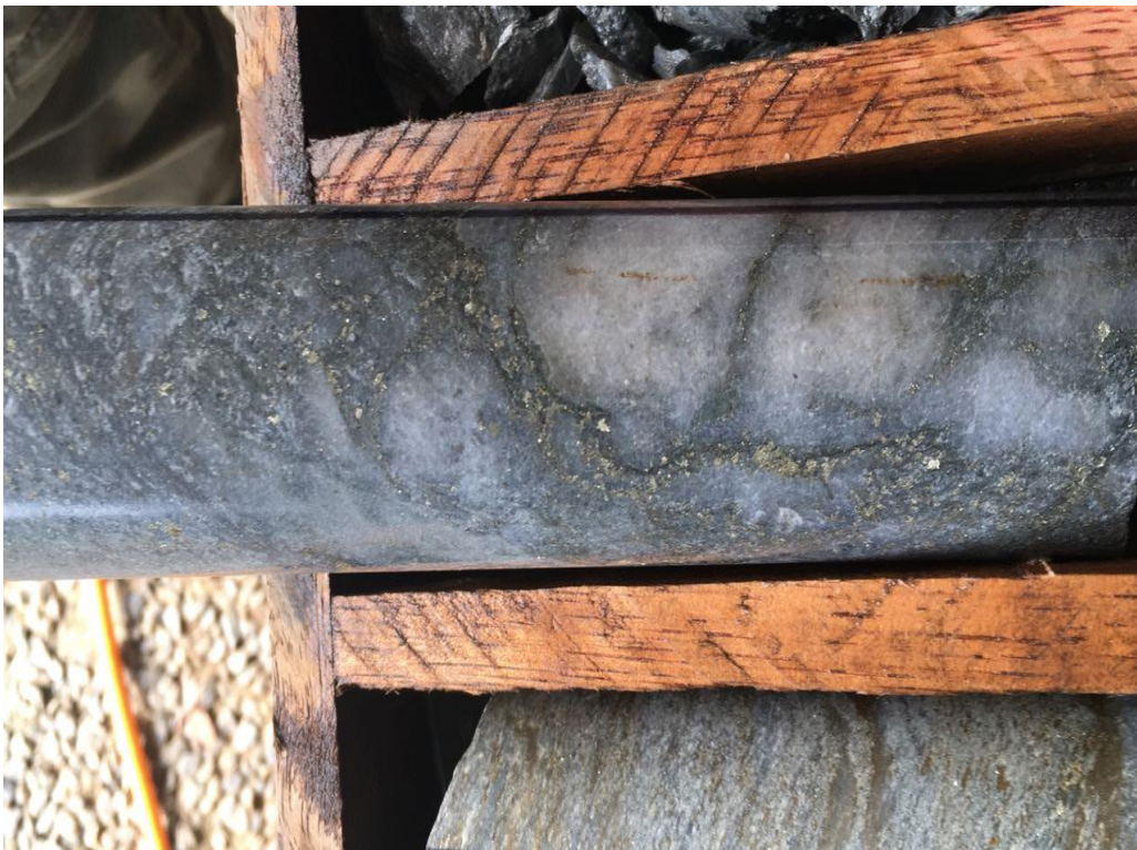
Photo 2: Detail of the sericitic alteration, with ASPY and PY in an intensive silicated zone at ANT_004, 158m depth
